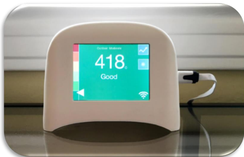
Speck sensor with data display
