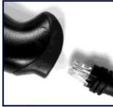
Step 3. Plug the USB end of the interface cable into an open USB port on your computer. The scanner should beep. If the scanner does not beep USB ports may be disabled on your computer. You will need to work with your internal desktop computer support personnel to enable your USB ports before continuing with this procedure.
