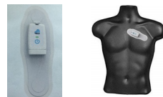
Figure 2. Wearable M5 Recorder used for ECG for Monitoring.
