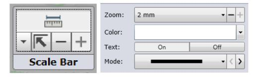
A scale bar options group was added to the headers of all the tabs as well. The scale bar options control contains options to allow the user to toggle on and off the scale bar, adjust the current level of the zoom, return the scale bar to its default position, change the bar's color, toggle on and off the unit text, and to change the display mode of the scale bar. Three display modes available are: bar, line, and ticks.
