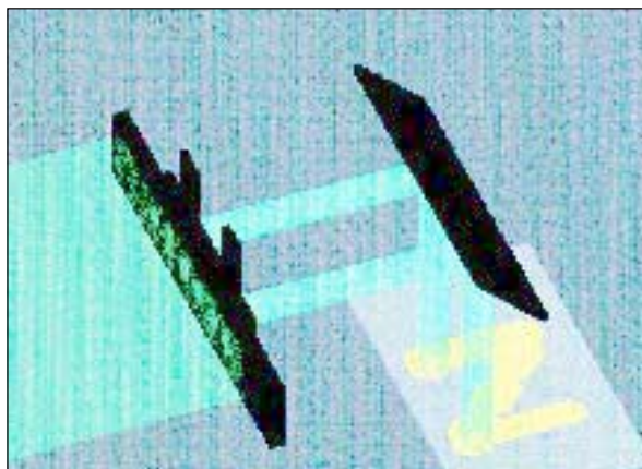
Figure 14. Representation of the Nidek EC-5000 excimer laser segmental small-area (1.0 mm) ablation system. The segmental ablation system has six apertures, 1.0 mm in diameter. Several apertures can be used simultaneously for more efficient treatment.
